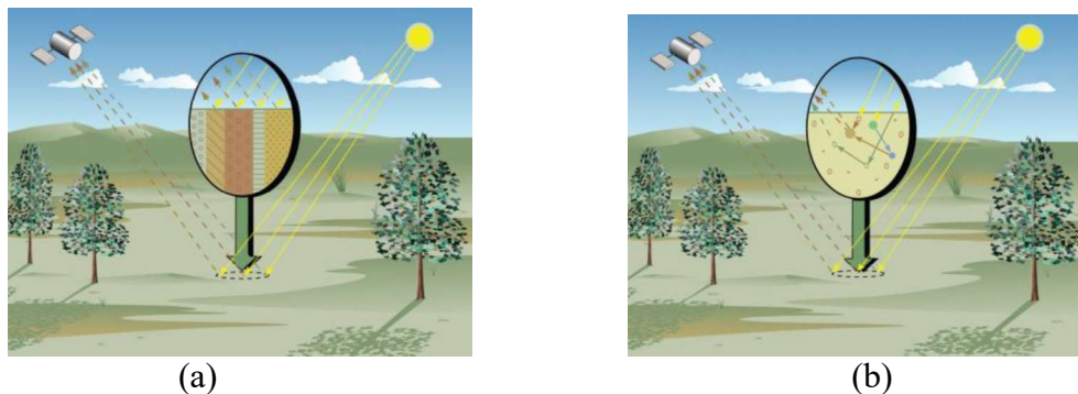
Figure 1: Two mixing models. (a) The linear mixing model assumes a well-defined checker board mixture of materials, with a single reflection of the illuminating solar radiation. (b) Nonlinear mixing models assume a randomly distributed, homogeneous mixture of materials, with multiple reflections of the illuminating radiation. (Adopted from Hapke, 1981)
